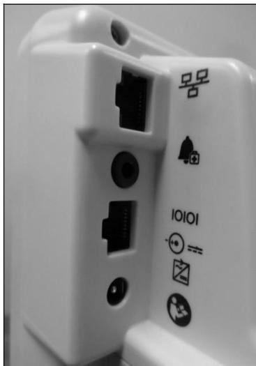
The top corner of the back of the Surveyor S12 and S19 contains the communication ports, an opening for the audio speaker as well as a connection for CO2 exhaust.
