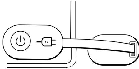
6. Connect the power button flex cable to J6 on the main board.
