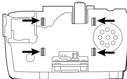
2. Remove the two Torx screws from the battery compartment and remove the battery board.
