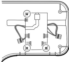
3. Lift and remove the PCBA.
