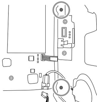
5. Pull the module handle assembly USB cable through the access hole in the power panel.
