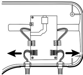
3. Lift and remove the handle cables from the front handle housing.
