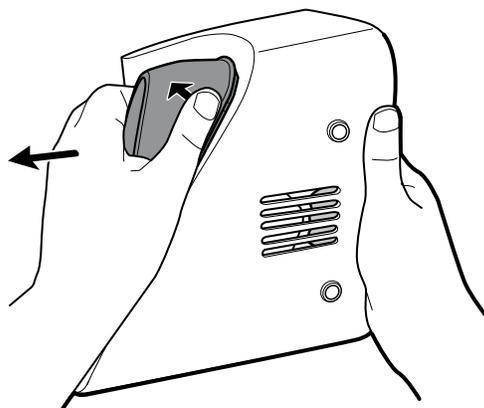
2. When the dock is completely loose, remove it from the housing.
