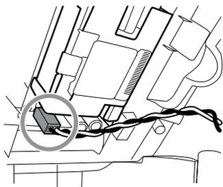
6. Separate the chassis from the front housing enough to make the AC power harness ground connection reach the dual spade connector.
