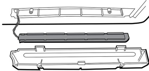
3. Remove the light bar from the light-bar cover.
