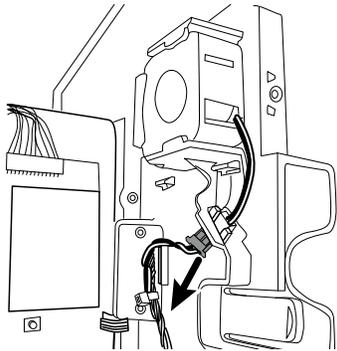
2. Press the flanges on the sides of the fan harness connector and separate the fan connector from the power panel.
