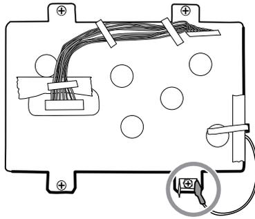
3. Remove the four large Phillips (shoulder) screws that secure the LCD frame along with the dual spade connector.
