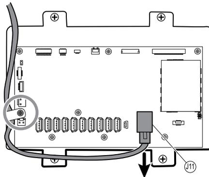
5. Remove the four large Phillips screws that mount the LCD to the housing.
