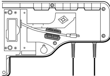
4. Remove the four large Phillips screws while supporting the end of the handle module assembly.
