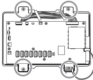
6. Carefully lift the LCD and the attached main board from the housing.
