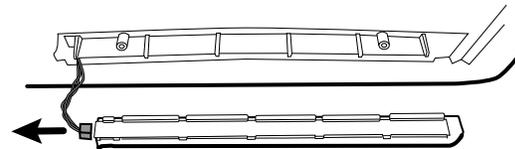
5. If replacing the light-bar board, remove the light-bar board from the light bar by sliding the board out from the connector end.
