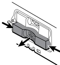
6. Disconnect the USB cables from the rear of each module.
