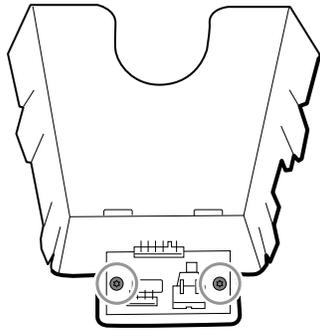
3. Secure the new battery board to the battery compartment with two Torx screws.
