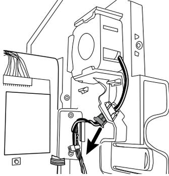
2. Disconnect the two harness connectors from the battery board.
