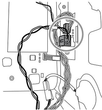
3. Disconnect the speaker connector wire.
