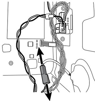
4. Remove the two Torx screws that attach the power panel to the front housing and slide the power panel out of the housing.
