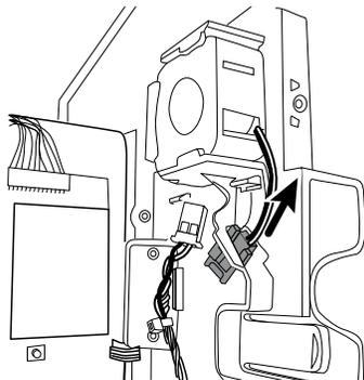
3. If you are removing the fan, slide the fan up and remove.
