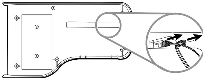
2. Push in the snap tabs and remove the cradle assembly by pushing outward.
