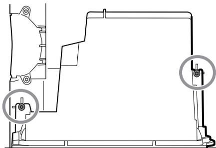
3. Remove the module well from the front housing. Remove the attached USB cables if necessary.
