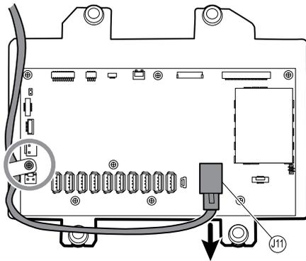
3. Remove the seven small Phillips screws that secure the main board to the LCD frame.
