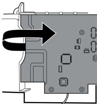
6. If replacing the communications board, remove the radio board as described in "Remove the radio board and antenna."
