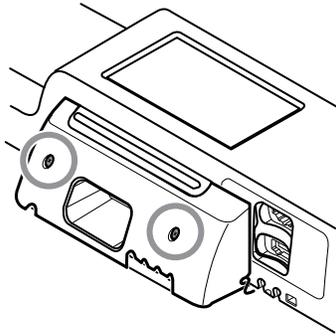
8. Remove the wall anchor screws using a #2 Phillips screwdriver.
