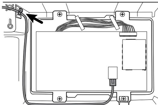
3. Remove the seven small Phillips screws that secure the main board to the LCD frame.
