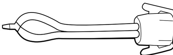
The blood pressure Y-tube is a piece of custom test equipment that connects the device to the test setup. The Y-tube is composed of a modified blood pressure hose and a Y-type fitting. Follow these instructions to create a Y-tube.
