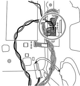
3. Disconnect the speaker connector wire.
