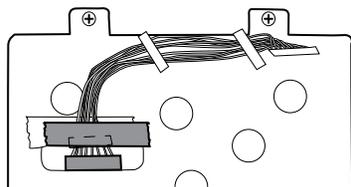
2. Disconnect the LCD ground wire from the dual spade connector.
