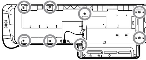
3. Remove the two Torx screws securing the client USB connector to the housing, and then disconnect and remove the cable.
