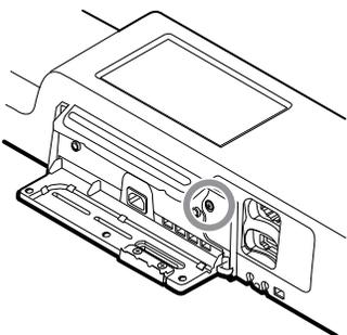
**Note** The modules fit tightly in the housing but can become loose over time. Support the modules to prevent them from falling out as you remove the module cover.
