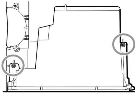
3. Remove the module well from the front housing. Remove the attached USB cables if necessary.
