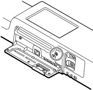
**Note** The modules fit tightly in the housing but can become loose over time. Support the modules as you remove the module cover.
