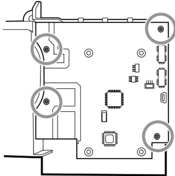
4. Lift the communications board from the chassis.
