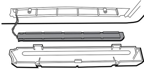
3. Remove the light bar from the light-bar cover.
