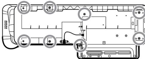
2. Remove the two Torx screws securing the client USB connector to the housing, and then disconnect and remove the cable.
