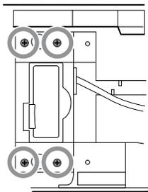
5. Lift the handle module assembly up and away from the main assembly while guiding the USB cable through the slotted opening.
