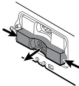
6. Disconnect the USB cable from the rear of the module.
