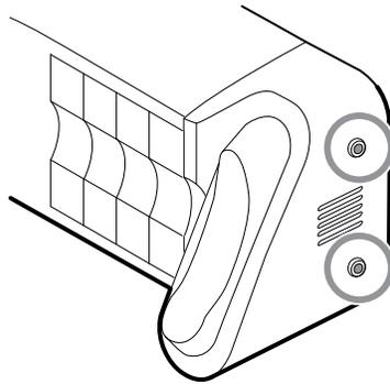
3. Remove the end cap or thermometer housing by sliding the piece away from the wall and then to the right.
