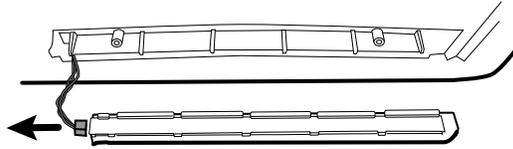
5. Remove the light-bar board from the light bar by sliding the board out from the connector end.
