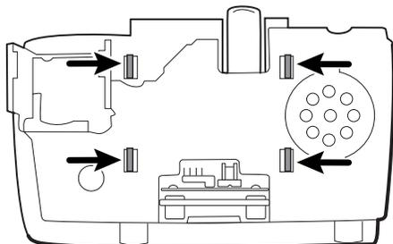
2. Remove the two Torx screws from the battery compartment and remove the battery board.
