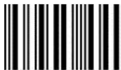
2. If "156544" appears on the host I2of5 symbology is enabled, no further action is required. If "156544" fails to appear on the host I2of5 symbology is not enabled, follow the procedure below to enable.
